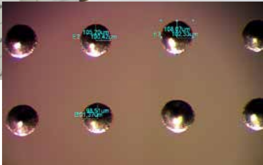
Dispensed droplets with ~190µm drop diameter
