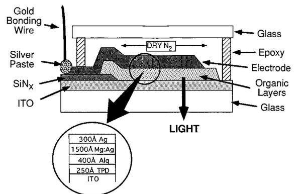
FIG. 1. Schematic side view of an encapsulated OLED.
