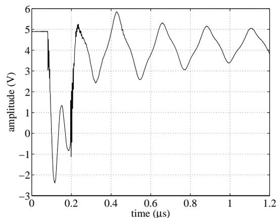
**Figure 5: Excitation of a 12 mm diameter PZ27 disc through a 7 cm long coaxial cable.**
