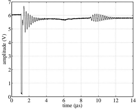
**Figure 3: Oscilloscope trace of excitation and received echo.**
