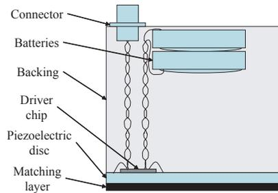
**Figure 6: Proposed sensor design with batteries cast into the backing material.**
