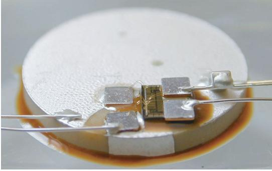
**Figure 1:** The driver chip mounted on a 16 mm diameter 1 MHz PZ27 disc. The 25  $\mu\text{m}$  gold bond wires are visible in the picture.
