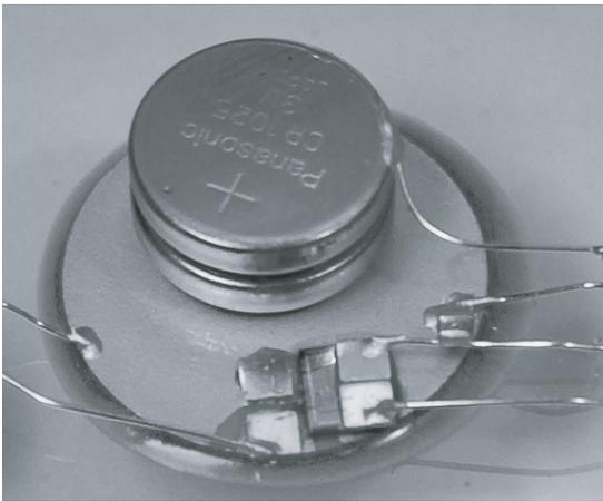
**Figure 2:** The driver chip mounted on a 16 mm diameter PZ27 disc together with two lithium button cell batteries.
