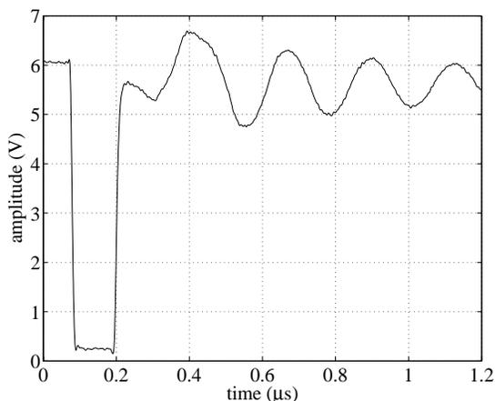
**Figure 4: Oscilloscope trace of excitation pulse generated with the driver stage mounted directly at the 16 mm PZ27 disc.**
