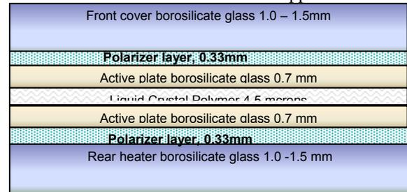
Figure 8. Schematic of LCD glass sandwich
