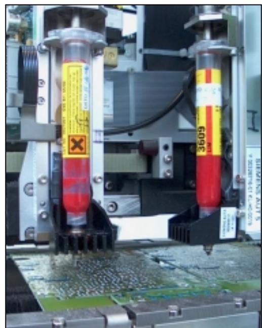
To make perfect adhesive dots, the PCB support must hold the PCB in a locked position and absolutely parallel to the X and Y-axis. The PCB support must be designed for both flexibility and fast change over. To ensure the necessary dispensing accuracy and repeatability an automatic vision alignment system using PCB fiducial marks combined with a closed-loop servo system must be included. These systems correct the program coordinate data to align with the PCB.
