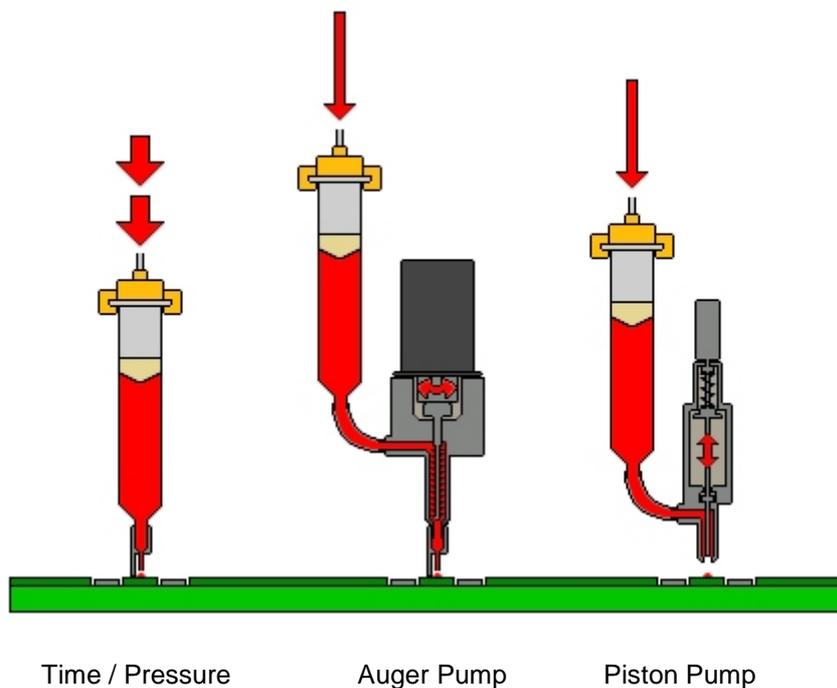
The adhesives' deposit and shape are determined by different factors, such as adhesive viscosity, adhesive supply pressure, dispense time (time / pressure system), auger rotation (auger system), number of piston strokes (piston system), dispense rate and nozzle standoff height.
