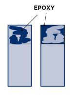
COHESIVE FAILURE Typical failure mode of an epoxy ADHESIVE FAILURE
