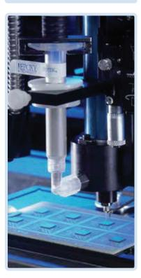
Commonly, customers will purchase two-component epoxies premixed and frozen in syringes for automated dispensing. This removes the weighing step and ensures that material has already been properly mixed for two-component systems.
