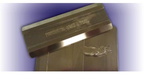
The resultant thin coating or film on the block is then visually inspected for any lumps or non-uniformites on the surface of the coating. Any visual observations can also be read using the scale along either side of the block. This scale can be read in Hegman units (dimensionless), micrometers or mils.
