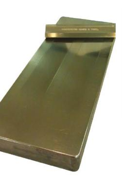
For wet particle analysis, a Hegman Gauge (sometimes referred to as a grind gauge) is frequently used to determine the fineness of the grind and to analyze different types of particles within an epoxy matrix. The test involves a flat, stainless steel block with two top channels, decreasing slightly in depth from one end to the other. The channel depth begins at 100µm and decreases to zero, with a corresponding scale on either side.
