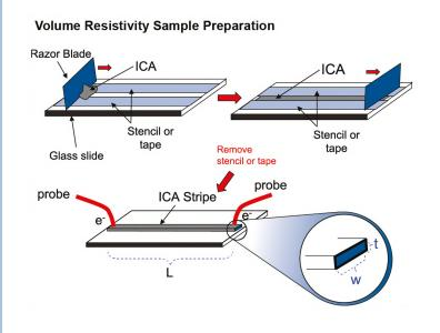
Once the sample has been prepared and cured, the two probes of a voltmeter are applied to the ends of the stripe to measure the resistance across the sample. Volume resistivity is then calculated according to the following equation:
